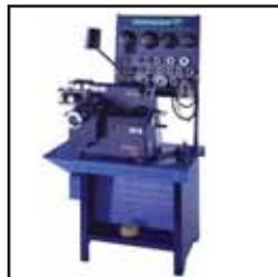
Combination brake lathes for rotors, drums, and flywheels.
