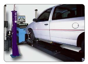
Alignment level at 21 safety locked working heights.
